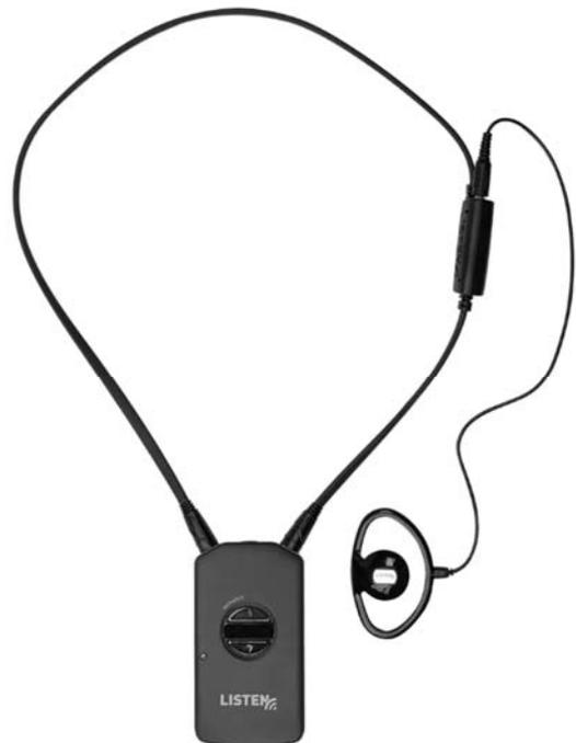
IR receiver with Neck loop lanyard and earpiece
