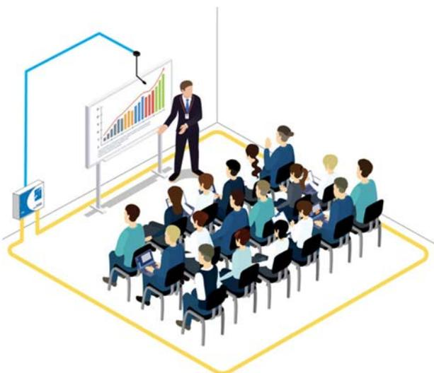
A typical perimeter type loop system
